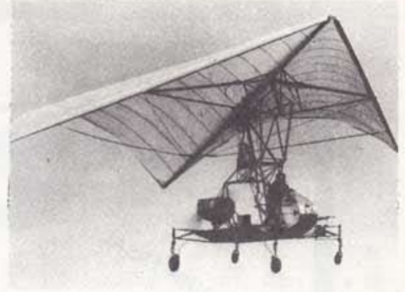
Flexwing with cowled engine and no rudder.
