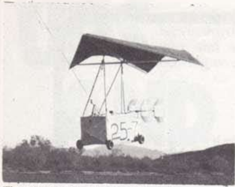
The pilotless air cargo tow glider had an automatic device to flare the machine for landing.
